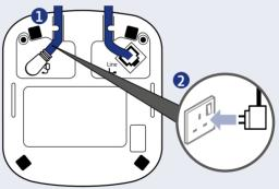
The telephone line cord is pre-installed but **don't** plug the other end into the wall socket yet.
