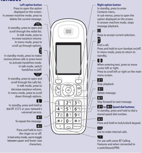
The answer machine handset controls on buttons 2<sup>4</sup> 4<sup>4</sup> 5<sup>4</sup> and 6<sup>48</sup> will only work when a message is being played on the handset.
