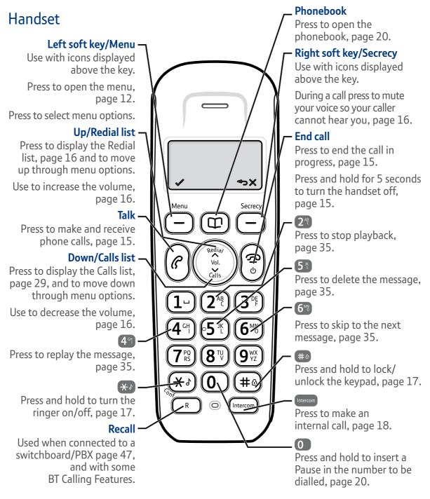
The answer machine handset controls on buttons 2<sup>4</sup> 4<sup>4</sup> 5<sup>4</sup> and 6<sup>48</sup> will only work when a message is being played on the handset, page 35.
