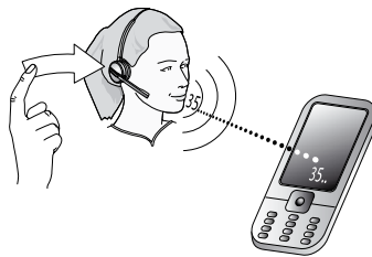
Figure 9: To use voice-activated dialing, tap the multifunction button and speak the appropriate voice tag
