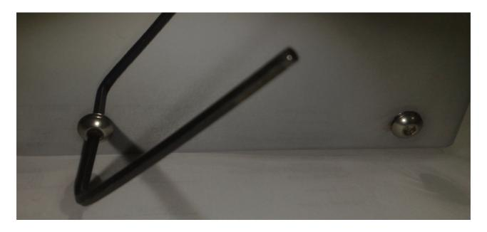
M4 securing screws being released with Allen Key
