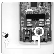
**3 -** Remove the jumper from the pins.
