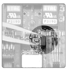
**2 -** Now locate the jumper, (a small black plastic square), there is only one jumper inside the Pico. It is located against the side of the smaller of the two telephone line connectors and it is marked JP1
