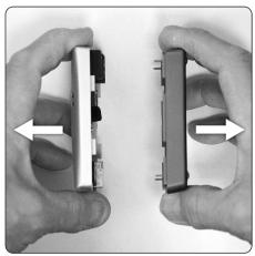
**1 -** Carefully open the Pico by disconnecting the blue and the gray parts, this should be easy.
