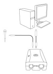
After connecting the Pico to the telephone line or microphone, it can be connected to the PC.
