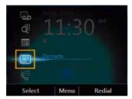
2. From the Contacts screen, use the up and down arrow buttons on the phone to select the contact, and then select **Call**.
