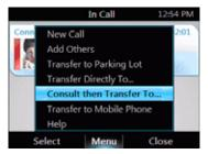
2. Enter a number or select a contact, and, when the contact accepts, select Complete Transfer.
