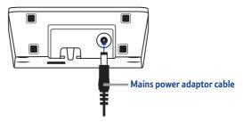
Then plug the other end into the mains wall socket but don't switch the power on at the wall socket yet.
