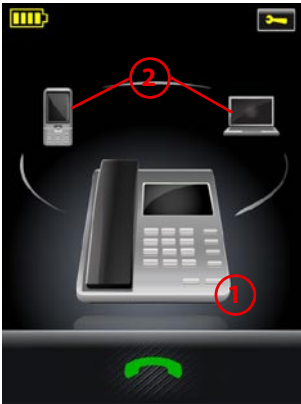
Figure 18: The current target phone is indicated by the large icon on the touchscreen; change the target by touching on one of the other icons
