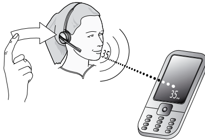
Figure 23: To use voice-activated dialing, tap the multifunction button and speak the appropriate voice tag
