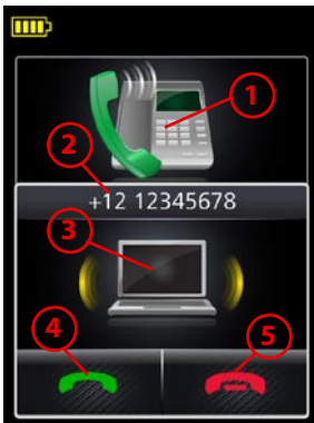
Figure 35: Touchscreen information and options for handling call collision
