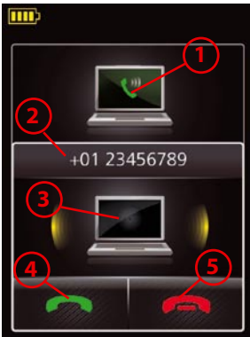
Figure 36: Touchscreen controls for managing call waiting when a new call arrives
