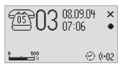
The display shows a clock as the symbol for activated timer. The timer sets the current functional status.
