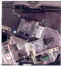
Coins are inserted without force into the mechanism, which has the capability of learning future coin changes. A bulk escrow provides prepayment coin storage, and subsequent cashing or refund of coins.
